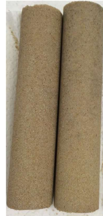
Sand treated with PropCure Coating forms a consolidated core
